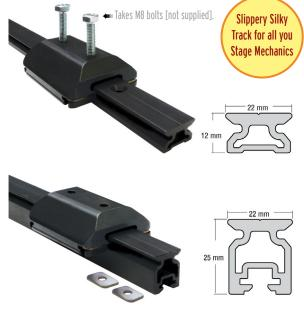
Ball Bearing Cars and Track These super smooth freerunning cars and tracks are used in everything from sliding seats to window washing apparatus and from exercise machines to acrobatics. Loads move virtually free of any friction. The recirculating Delrin ball bearings are held captive so the cars can be easily removed from the tracks.
